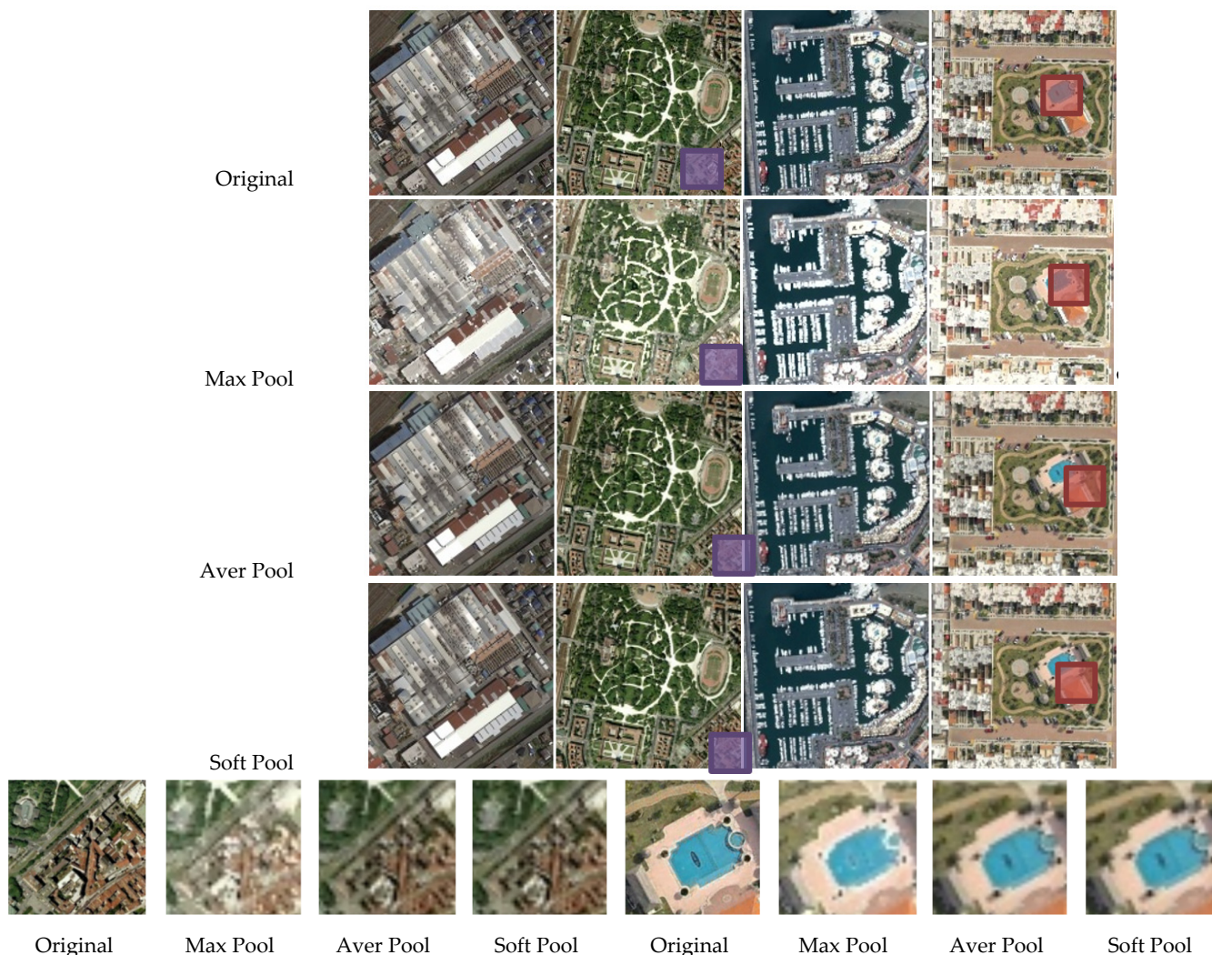
Figure 8. The effects of different pooling methods. The bottom row is the zoom area of the above image.
