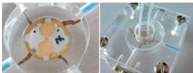
Figure 1. Left: Quartz crystal microbalances (QCM) positioned on the copper electrode wires. Right: Placement of the lid with inlet and outlet on top of the sensor.
