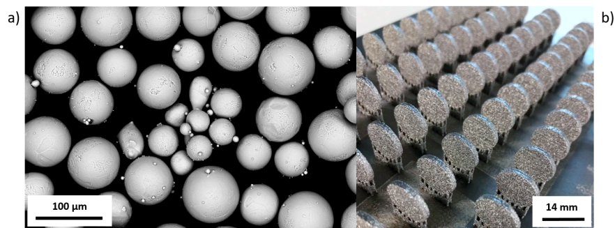
Figure 1. (a) SEM image of Ti6Al4V ELI (Arcam AB) powder particles. (b) View on the platform with EBM-manufactured pellets.
