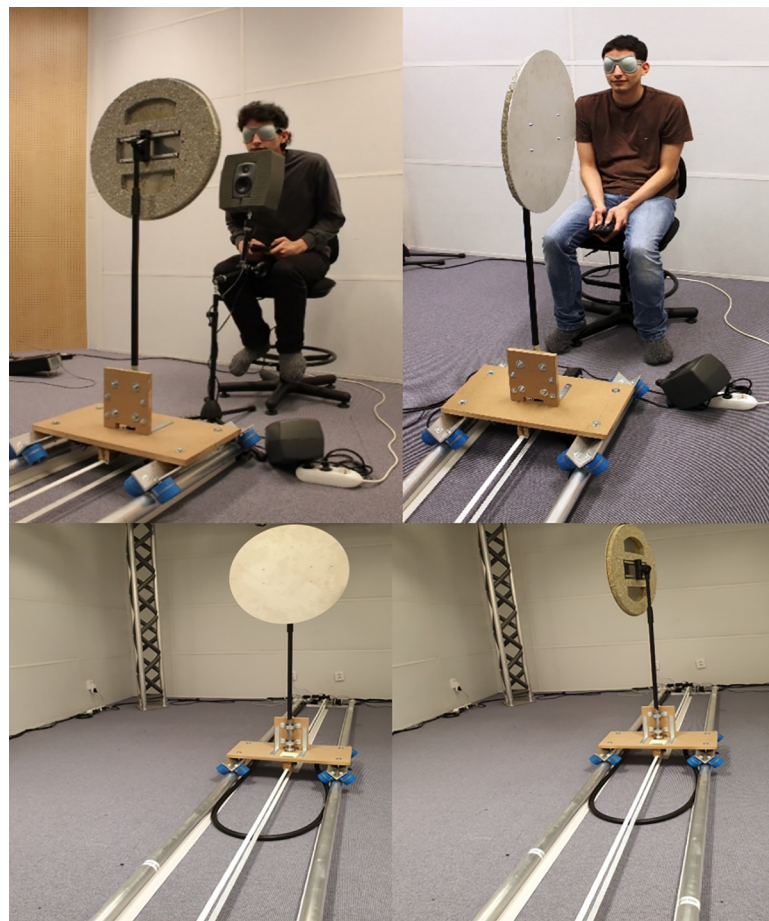
Fig 1. The Echobot. In a reflecting position (upper left picture) and in a non-reflecting position (upper right picture). The blindfolded participant responded using a wireless keyboard. The loudspeaker in front of the participant, covered with a sound absorbing material, generated the echolocation click in the loudspeaker experiment, and worked as a chin rest. In the vocalization experiment, the participant generated their own signals (upper right picture). In both experiments, the loudspeaker on the floor played a masking sound while the Echobot was moving and provided auditory feedback (“right” or “wrong”) after the participant had responded. The Echobot moved along a 4 m long rail. In the present setup, it could stop at distance between 0.7 and 3.9 m from the participant. After it stopped, the disk was either rotated to a reflecting position (lower left picture) or non-reflecting position (lower right picture). The individual in these pictures, who is one of the authors, has given written informed consent (as outlined in PLOS consent form) to publish these images.
