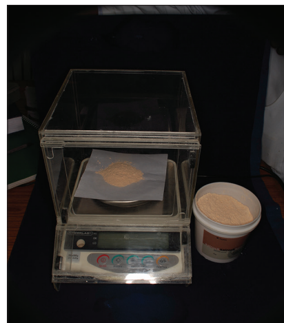
Figure 4: Electronic measuring balance used for weighing dental stone
