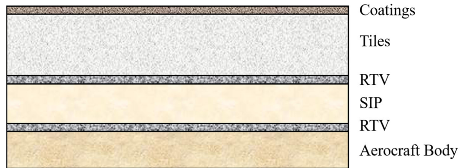
Figure 5. Connection method between the thermal protection tiles and the spacecraft.
