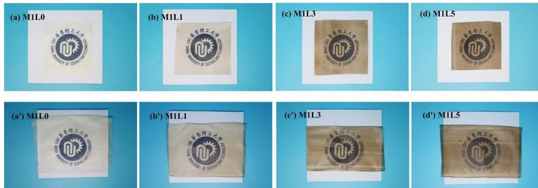
**Figure 7.** Photos of starch/PBAT composite film before and after UV aging. Before: (a) M1L0, (b) M1L1, (c) M1L3, (d) M1L5; After: (a') M1L0, (b') M1L1, (c') M1L3, (d') M1L5.
