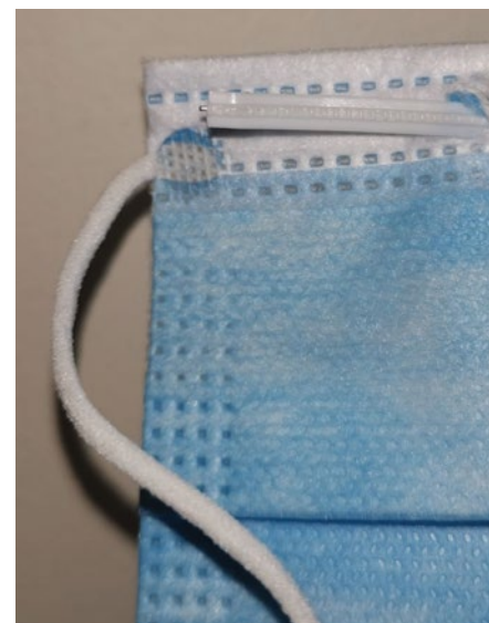
Fig. 3 Fluid resistant surgical face mask – demonstrating the aluminium metal wire extruded from its superior horizontal margin
