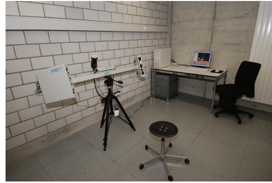
FIGURE 1: 3dMDface system (3dMD Inc., Atlanta, GA, USA) as utilized for image acquisition; desktop PC performing necessary calculations and storing data.
