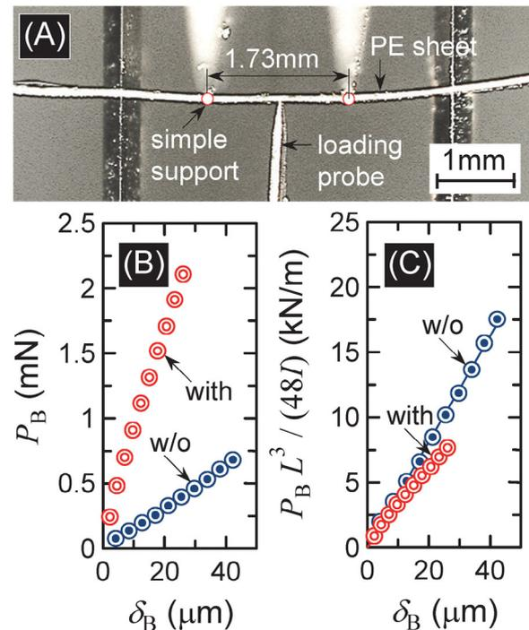
**FIGURE 4** (A) Experimental setup for three-point bending test of polyethylene (PE) sheet. (B)  $P_B$  versus  $\delta_B$ , and (C)  $P_B L^3 / (48I)$  versus  $\delta_B$  of the PE sheet with and without nail strengthener (sample H1).
