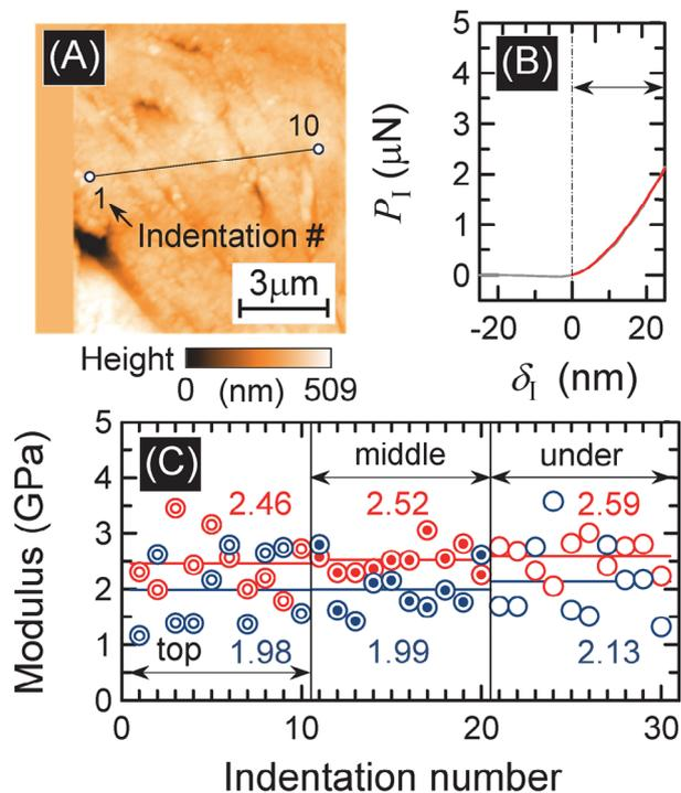
**FIGURE 2** Results of nanoindentation (sample N3): (A) AFM image of cross-section of the top plate of the nail sample. (B) Relationship between  $P_1$  and  $\delta_1$  at the position (indentation #6). (C) Young's moduli at each indentation number before (red) and after (blue) softening treatment for 1 h.
