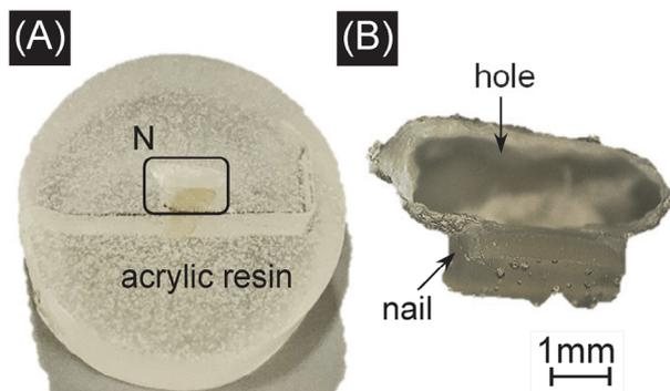
**FIGURE 1** (A) Photograph of nail sample, where the nail is embedded in acrylic resin. (B) Details of *N* in (A), where the hole is introduced on the top surface of the nail for softening treatment.
