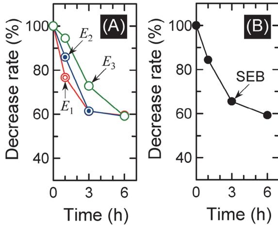
**FIGURE 3** Results of softening treatment: (A) Decrease rate of Young's modulus of each plate against the time for softening treatment, and (B) that of SEB. SEB, structural elasticity for bending deformation.
