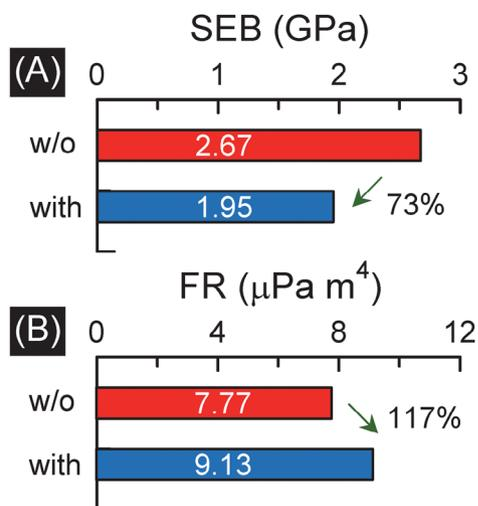
**FIGURE 5** Comparison of (A) SEB and (B) FR of the nail with and without nail strengthener on top of the nail surface. The thicknesses of the nail and nail strengthener were assumed to be 432.4 and 54.4  $\mu\text{m}$ , respectively. SEB, structural elasticity for bending deformation.
