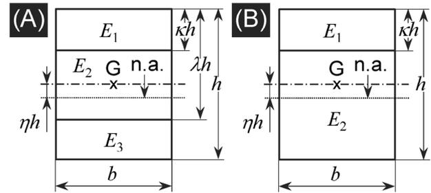
**FIGURE A1** (A) Three-layered and (B) two-layered structures having rectangle cross-sections. The height and width of the structure are  $h$  and  $b$ , respectively.
