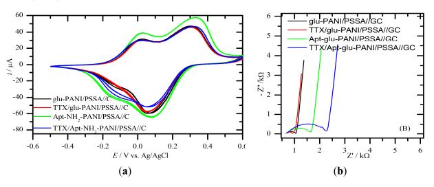
**Figure 5.** (a) CVs and (b) EIS spectra of TTX aptasensor (Apt-NH<sub>2</sub>-glu-PANI-PSSA//C) and the control sensor (glu-PANI/PSSA//C) before and after 30 min exposure to 5  $\mu$ M TTX standard solution in NaOAc buffer (0.1 M, pH 4.8).
