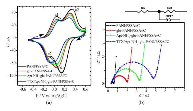
**Figure 4.** CVs (**a**) and EIS spectra (**b**) of TTX aptasensor and its electrode materials. Conditions: NaOAc buffer (0.1 M and pH 4.8); initial CV scan direction is cathodic; and EIS's E = 0.010 V and f = 100 mHz–100 kHz. The equivalent circuit on top of (**b**) was used to fit the Nyquist plots ( $R_s$ ,  $R_{ct}$  and *CPE1* are solution resistance, charge transfer resistance and constant phase element, respectively).
