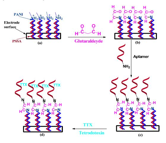
**Figure 1.** Schematics for the development of the TTX aptasensor: (**a**) electrodeposition of PSSA-doped polyaniline onto the carbon electrode; (**b**) glutaraldehyde-functionalization of PANI/PSSA film; (**c**) immobilization of NH<sub>2</sub>-aptamer on glu-PANI/PSSA/GC; and (**d**) TTX detection.
