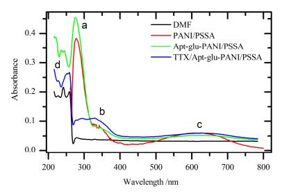
**Figure 3.** UV-Vis spectra of PANI/PSSA, Apt-NH<sub>2</sub>-glu-PANI/PSSA, and TTX-Apt-NH<sub>2</sub>-glu-PANI/PSSA composite materials dispersed in DMF.
