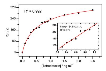
**Figure 6.** Calibration plot of the impedimetric TTX aptasensor (main graph); and the plot of the analytical linear range of the aptasensor (inset).
