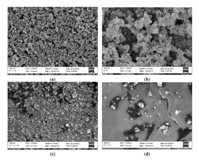
Figure 2. Scanning electron micrographs of (a) bare C-SPE; (b) PANI/PSSA//C-SPE; (c) Apt-NH<sub>2</sub>-glu-PANI/PSSA//C-SPE; and (d) TTX-Apt-NH<sub>2</sub>-glu-PANI/PSSA//C-SPE (where C-SPE is carbon screen printed electrode).
