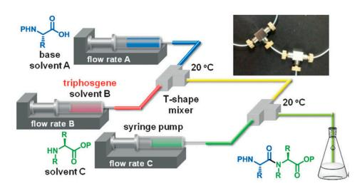
**Figure 1.** Microflow synthesis of peptides based on rapid and strong activation of carboxylic acids. Adapted with permission from Reference [13].
