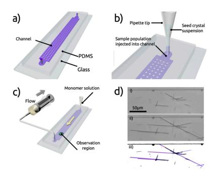
**Figure 3.** Microfluidics platform for the control of peptide self-assembly. (**a**) presentation of the microre-actor (multiple inlets and central chamber), (**b**) injection of seed crystals, (**c**) injection of a satu-rated solution of FF, (**d**) images via optical microscopy. With permission from Reference [32].
