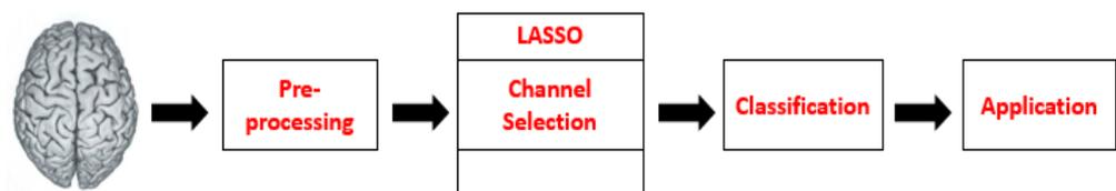
**Figure 2.** BCI system with LASSO-based sparse representation classification for channel selection.
