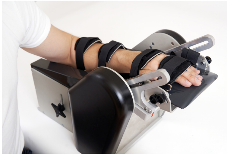
Fig. 1 NeuroFlexor measurement device. The NeuroFlexor instrument showing the position of the hand with the metacarpophalangeal joints in slight flexion and the fingers completely extended, and with the wrist axis of rotation aligned with the device. The instrument passively extends the wrist joint in a 50° range of motion with a starting angle of 20° of palmar flexion, and the movement is performed at controlled slow and fast velocities (5 and 236°/s, respectively)
