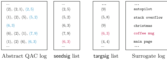
Fig. 2. The synthetic pattern generation process. Signatures of FinalP from the abstract QAC log are used to form the seedsig list, and the signatures from surrogate log form targsig list. A match between the signature (6, 3) in the seedsig list and in the targsig list might correspond to the target string “coffee mug”.
