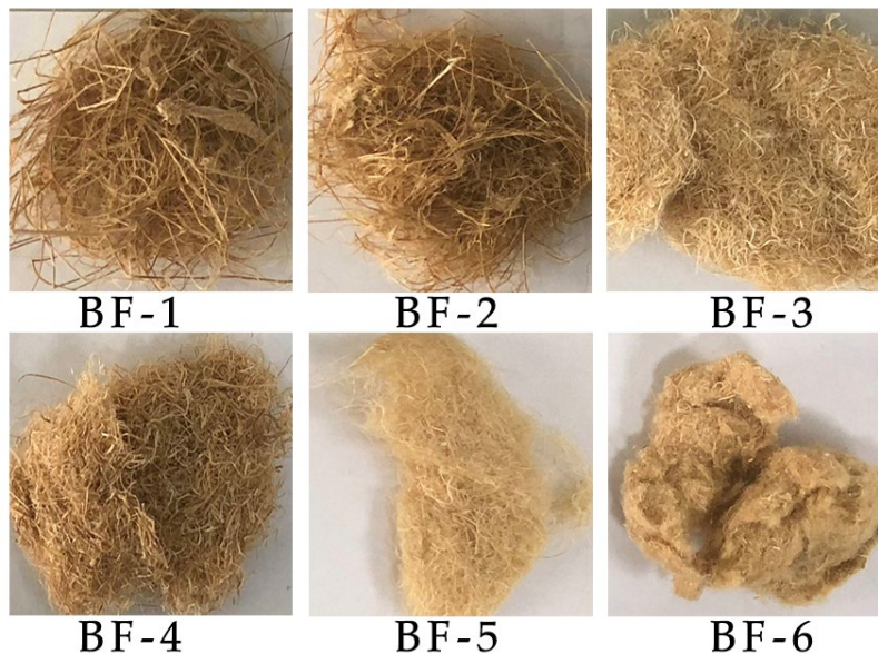
Figure 2. Macroscopic morphology of bamboo fibers with different opening times.
