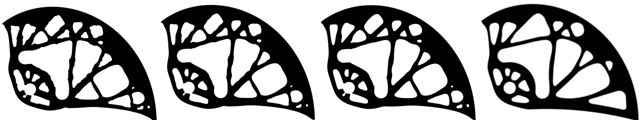
Figure 11. Cam shape after smoothing achieved by calculations using various values of polynomial degrees of k = 5, 10 , and 100 (from the left), and the optimal cam design with k = 250 (right).
