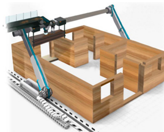
Figure 1. Schematic diagram of the autonomous rammed earth construction method.
