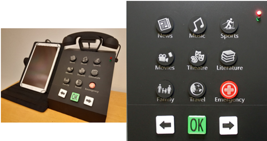
Fig. 3. TUI telephone (to the left) and its 12-key keypad (to the right)
