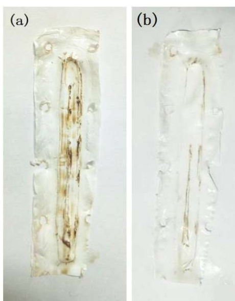
Figure 9. Pictures of as-prepared PVDF membrane (a) fouled membrane after fertilizer testing and (b) cleaned membrane rinsed with pure water.
