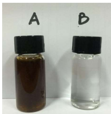
Figure 7. Images of original organic fertilizer sample (A) and MD permeate sample (B).
