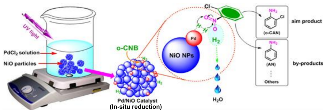
Scheme 1. Sketch map of the preparation of UV-light-irradiated Pd-based catalyst over NiO and the evaluation of its reactivity toward the o -chloronitrobenzene ( o -CNB) hydrogenation.
