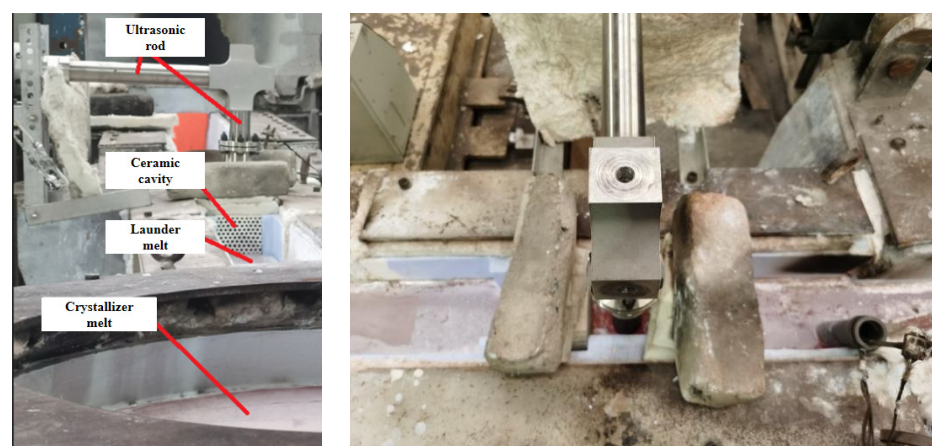
Figure 2. Online ultrasonic purification of launder melt site photo.
