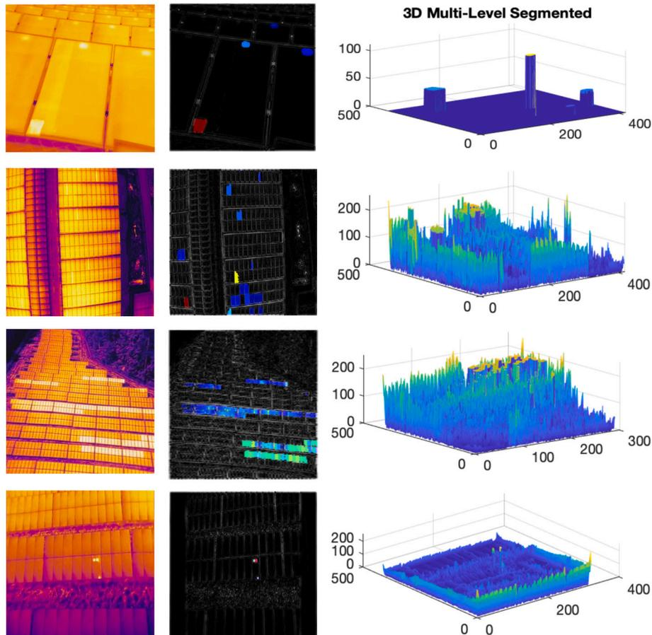
**Fig. 6.** Heat-map chart analysis of a deteriorated surface of 4 samples. Black areas indicate intact regions, while colored areas indicate higher levels of surface deterioration.
