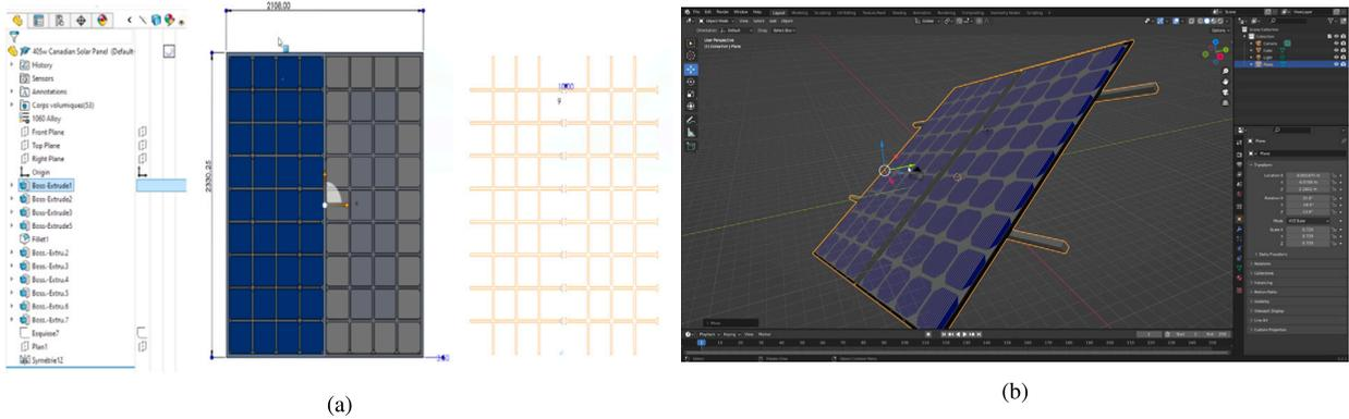
Fig. 3. (a) Solidworks conception, (b) PV Blender conception.
