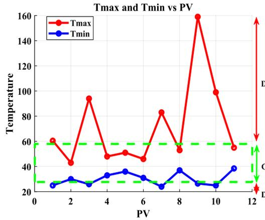
Fig. 4.  $T_{max}$  and  $T_{min}$  values for 11 PV panels, indicating which panels have deteriorated cells. Segmentation is necessary to accurately delineate the affected region and optimize performance.
