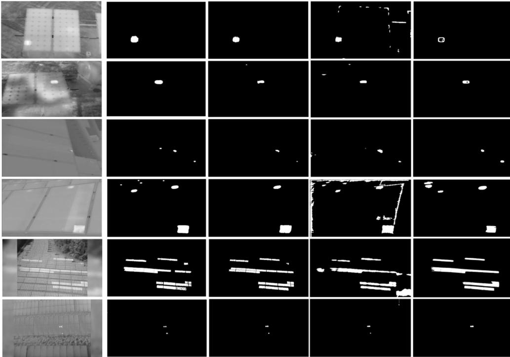
Fig. 5. Visual segmentation comparison of six image examples using various methods: Columns 1–5 respectively show the original image, ground truth, proposed, Weka, and SAM segmentation results.
