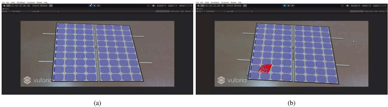
Fig. 7. PV and AR visualizations: (a) PV Augmented Reality visualization and (b) AR visualization of the PV deteriorated areas.
