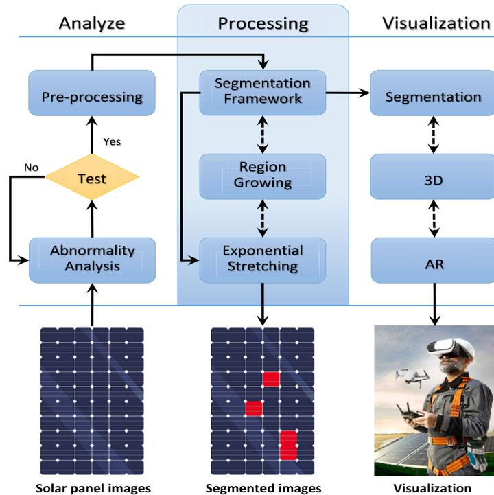
Fig. 1. Block Diagram of the methodology used for analyzing and visualizing deteriorated area in PV module.
