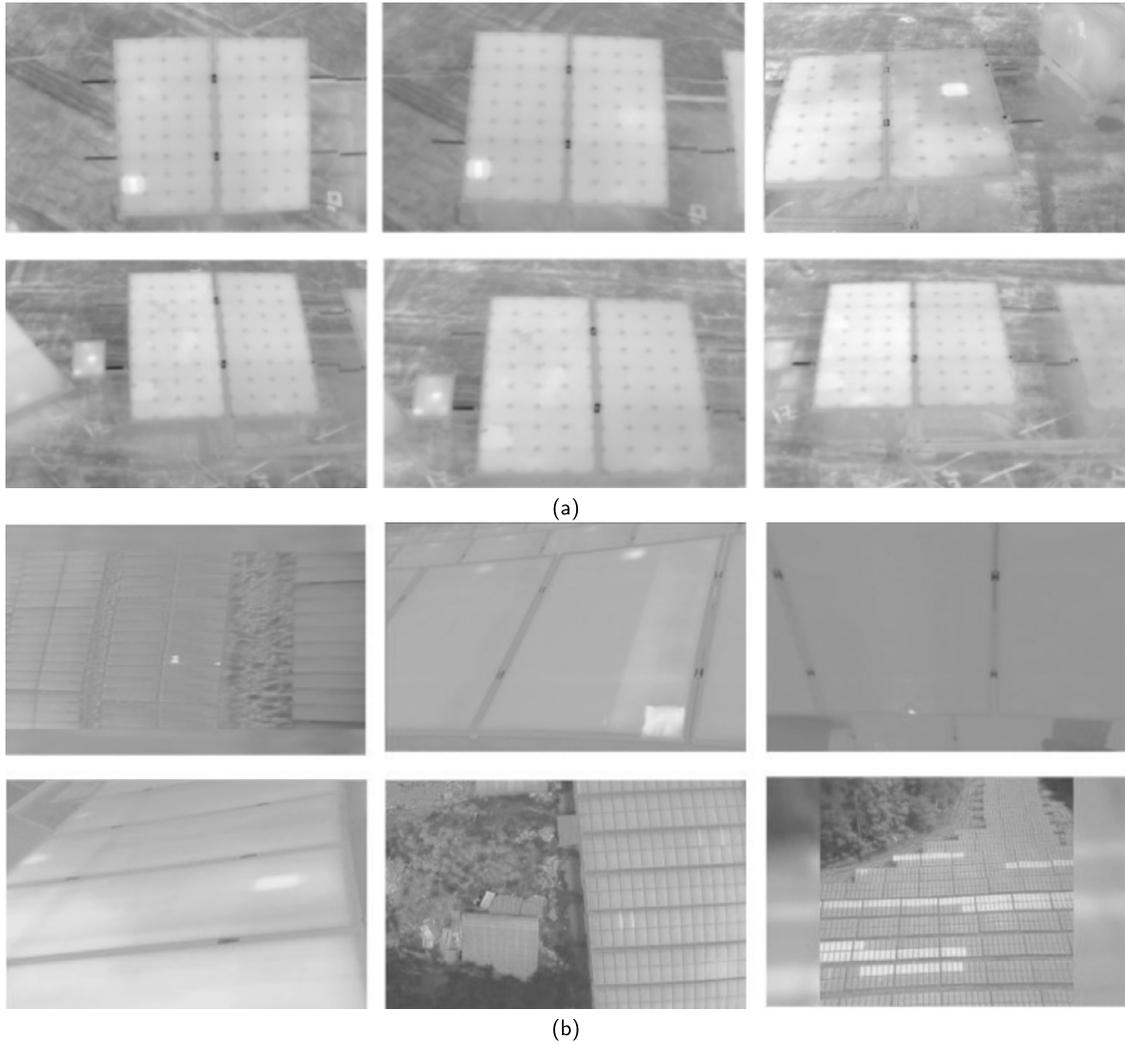
Fig. 2. Samples of abnormal and normal PV modules highlighting the distinct differences in visual appearance and potential defects on (a) Cali-Thermal Solar Panels and (b) Solar Panel Infrared Image Database.
