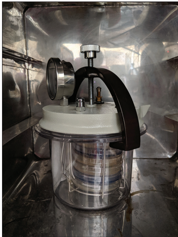
Figure 4: Ten microliters of the turbid growth streaked onto the selective culture media and incubated anaerobically using commercially available Gaspaks
