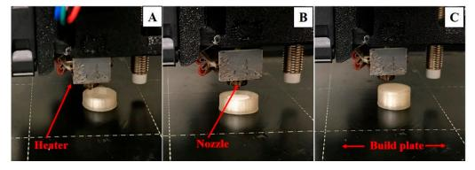
**Figure 4.** Eighty percent of the printed empty shell of a floating tablet (**A**), placement of a compressed tablet in the shell (**B**), and a completely sealed floating tablet (**C**).
