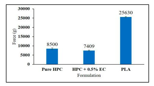
**Figure 3.** Force values of stiffness test of the hot-melt extruded filaments (error bars represent mean  $\pm$  S.D).
