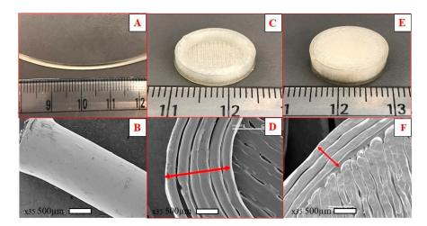
**Figure 6.** Digital images and representative SEM images of the hot-melt extrusion (HME) filament (**A**,**B**), the cross-sectional structure of the floating tablet showing shell (**C**,**D**), and surface morphology of a 100% infill 3D printed tablet (**E**,**F**).
