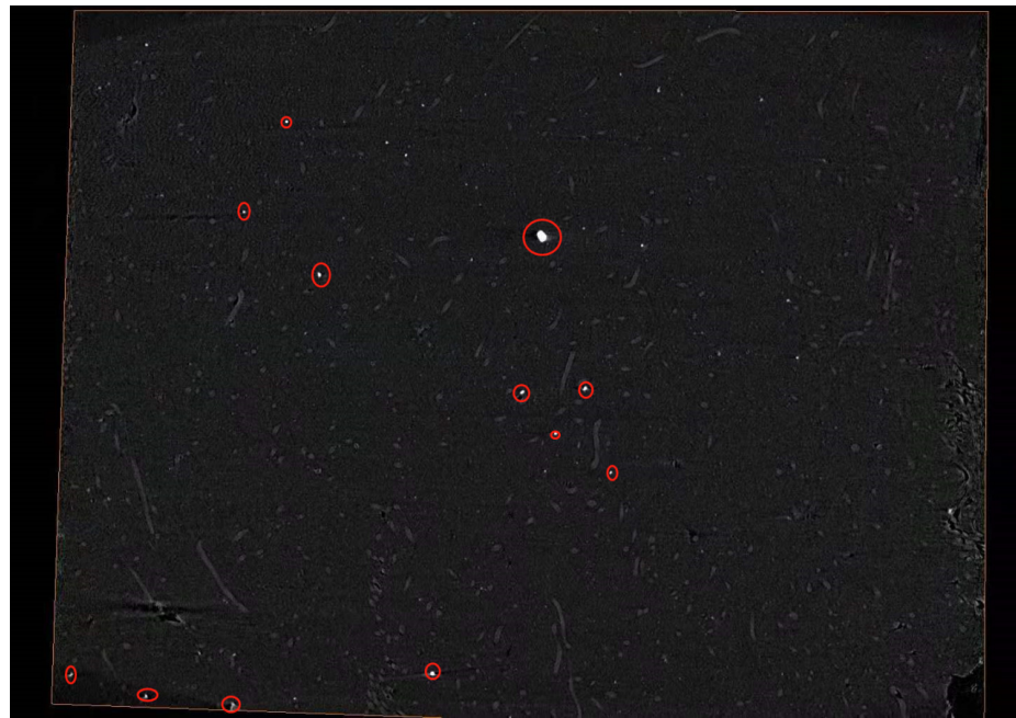
Figure 5. Slice image of a polyester-short-fiber-reinforced rubber composite sample before binarization treatment.
