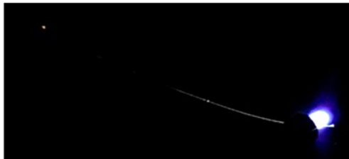
Supplementary Fig.47 | Demonstration of afterglow optical waveguide fiber.
