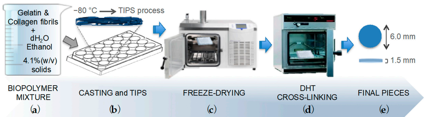
Figure 1. Nanofibrous biomaterial processing route: (a) Biopolymer mixture precursor composition; (b) pieces shaping and thermally induced phase separation (TIPS); (c) lyophilization process; (d) dehydrothermal treatment (DHT) cross-linking; (e) final pieces dimensions.
