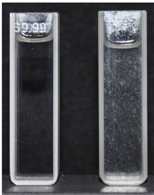
Fig. 2. Cells with IPA (left) and with the test solution (100 mg of the drug +20.0 ml IPA) (right).
