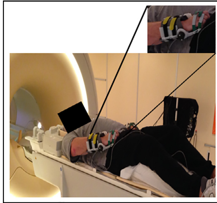
Fig. 1. Picture of experimental setup showing homemade MR-compatible goniometer attached to patient's wrist in MRI scanner room. Patient's wrist is at rest, corresponding to an angle of 0°.
