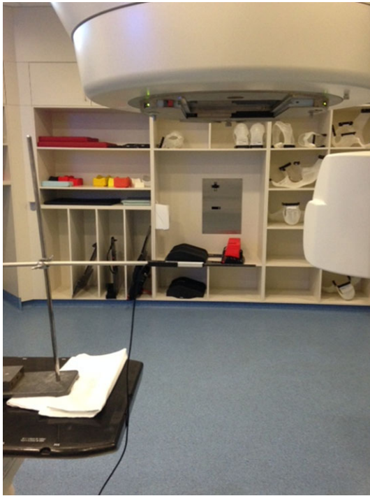
FIG. 3. Experimental setup for the measurement of \text{CTDI}^{\text{in-air}} . The 100-mm chamber was stepped in 100-mm increments to achieve the necessary integration length to capture the full dose profile. The chamber was held in place using a retort stand and rod. The chamber was extended from the couch a distance equal to half the total integration length to minimize scatter from the couch as specified by the IAEA. 15
