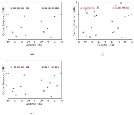
**Figure 11.** Joint estimation of DOA and CF, SNR = 10 dB, Q = 300, M = 30. (a) Proposed PJE algorithm with  $M_u = 10$ , (b) conventional JE algorithm with  $M_u = 10$ , (c) proposed PJE algorithm with  $M_u = 13$ . e: CF-known sources, e: CF-unknown sources,  $\times$ : estimated sources.
