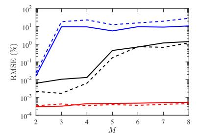
**Figure 4.** RMSE of DOA and CF estimation under different numbers of signals, SNR = 10 dB, Q = 300,  $M_u = 1$ . ——: RMSE of DOA with proposed PJE algorithm, ——: RMSE of CF with proposed PJE algorithm, ——: RMSE of DOA with conventional JE algorithm, ——: RMSE of CF with conventional JE algorithm, ——: CRB of DOA estimation, ——: CRB of CF estimation.
