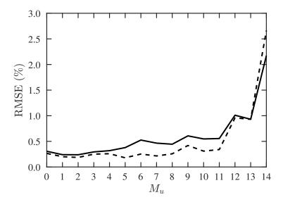
**Figure 6.** RMSE of DOA and CF estimation with proposed PJE algorithm, under different numbers of signals with unknown CF, SNR = 10 dB, Q = 300, M = 30. ———: RMSE of DOA, ---: RMSE of CF.
