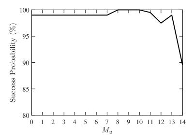
**Figure 5.** Success probability of DOA and CF estimation with proposed PJE algorithm, under different numbers of signals with unknown CF, SNR = 10 dB, Q = 300, M = 30.
