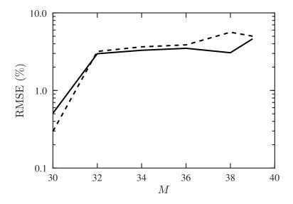
**Figure 8.** RMSE of DOA and CF estimation with proposed PJE algorithm, under different numbers of signal sources, SNR = 10 dB, Q = 300,  $M_u = 10$ . RMSE of DOA, --: RMSE of CF.
