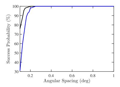
**Figure 13.** Success probability of DOA and CF estimation versus angular spacing, SNR = 10 dB, Q = 300, M = 3,  $M_u = 1$ . ————: proposed PJE algorithm, ————: conventional JE algorithm.
