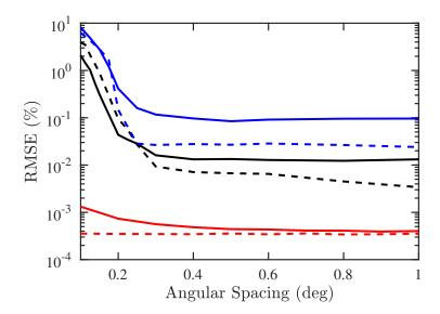
**Figure 14.** RMSE of DOA and CF estimation versus angular spacing, SNR = 10 dB, Q = 300, M = 3,  $M_u = 1$ . ——: RMSE of DOA with proposed PJE algorithm, ——: RMSE of CF with proposed PJE algorithm, ——: RMSE of DOA with conventional JE algorithm, ——: CRB of CF with conventional JE algorithm, ——: CRB of DOA estimation, ——: CRB of CF estimation.
