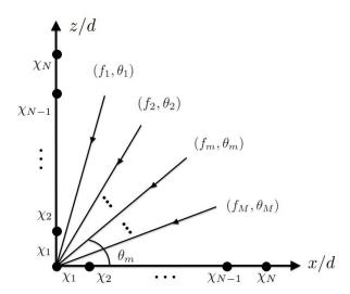
**Figure 1.** Orthogonal CPAs deployed along x and z axes, respectively, to estimate DOAs of M sources.
