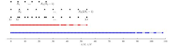
**Figure 2.** Configuration of CPA( $N_1$ ,  $N_2$ ),  $N_1 = 5$ ,  $N_2 = 6$ , **■**: first ULA at spacing  $N_1d$ , **△**: second ULA at spacing  $N_2d$ , •: physical array of CPA ( $N_1$ ,  $N_2$ ), •: second-order virtual array, ×: second-order holes, •: fourth-order virtual array, ×: fourth-order holes.
