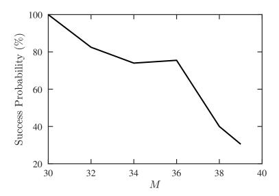
**Figure 7.** Success probability of DOA and CF estimation with proposed PJE algorithm, under different numbers of signal sources, SNR = 10 dB, Q = 300,  $M_u = 10$ .
