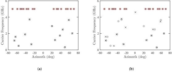
**Figure 10.** Joint estimation of DOA and CF with proposed PJE algorithm, (**a**)  $M_u = 13$  and (**b**)  $M_u = 14$ , SNR = 10 dB, Q = 300, M = 30. •: CF-known sources, •: CF-unknown sources, ×: estimated sources.
