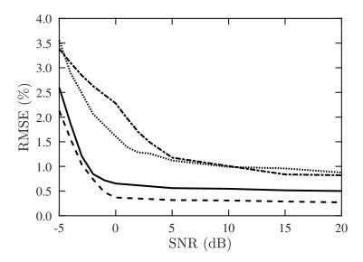
**Figure 12.** RMSE of DOA and CF estimation versus SNR, with proposed PJE algorithm, Q = 300, M = 30. ——: RMSE of DOA with  $M_u = 10$ , ---: RMSE of CF with  $M_u = 10$ , ---: RMSE of DOA with  $M_u = 13$ . ...: RMSE of CF with  $M_u = 13$ .
