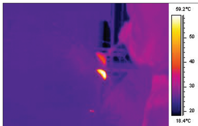
Figure 4: Calibrated infra-red thermal image during reaming on the sawbone model
