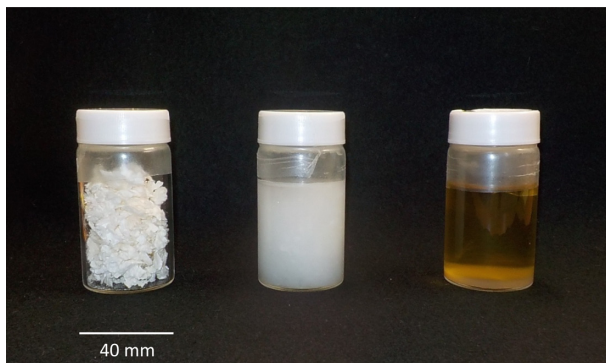
Fig. 1. Paper bedding (left), paper bedding dispersed in water (center), and paper bedding dissolved after hydrolysis (right).
