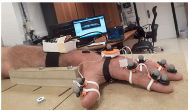
Fig. 7. The motion capture algorithm being tested with the Vicon Motion System.
