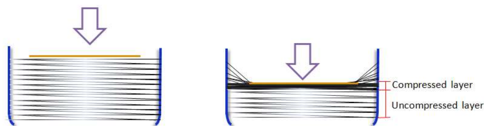
Figure 4. Schematic evolutions of the CB@PU network during continuous compressive deformation.
