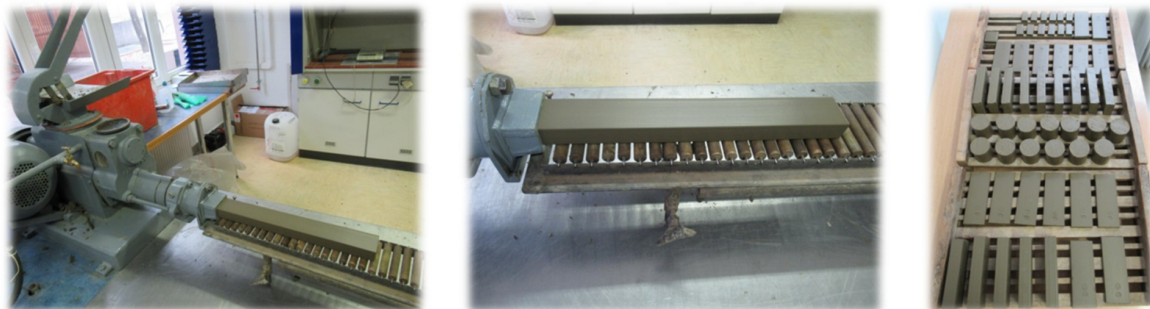
Figure 5. Sample preparation with a de-airing extruder.
