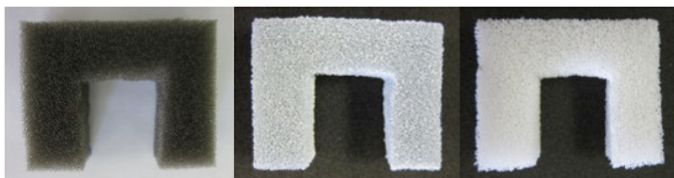
Figure 2. Representative stereo microscope (AmScope; SM-2TZ-M) images (x4) of a 80 ppi sized PU sponge (left), HA coated and dried BMT (middle), and sintered BMT (right). (Dimension: 3 cm in height x 4 cm in length x 1 cm in width). Please click here to view a larger version of this figure.
