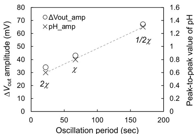
**Figure 2.** Peak-to-peak potential and pH (amplitude) for oscillation period computed on the basis of Figs. 1 and S2. The concentration  $\chi$  of the BZ solution was controlled to  $1/2\chi$ ,  $\chi$ , and  $2\chi$ . The oscillation periods,  $\Delta V_{\text{out}}$ , and  $\Delta\text{pH}$  were averaged in the limited range of about 5 min. Each standard error shows  $<0.3$  s for the oscillation periods,  $<0.5$  mV for  $\Delta V_{\text{out}}$ , and  $<0.01$  for  $\Delta\text{pH}$ .
