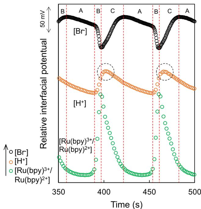
**Figure 3.** Self-oscillation behaviors of  $[H^+]$ ,  $[Ru(bpy)^{3+}/Ru(bpy)^{2+}]$ , and  $[Br^-]$  based on relative interfacial potential. The durations of Processes A, B, and C based on the FKN mechanism (Table S2) are delineated by the dotted lines (red). The dotted circle (black) shows the position of the peak  $[H^+]$ .
