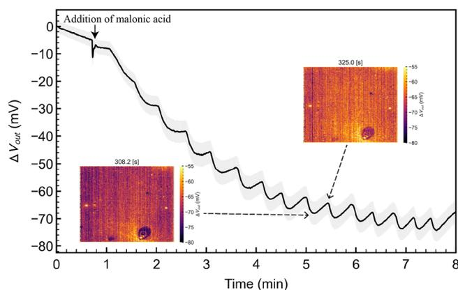
**Figure 4.** pH oscillation behavior on arrayed-gate ISFET sensor.  $\Delta V_{\text{out}}$  was output for pH analysis. The grey band around the line graph shows the standard errors for the  $256 \times 256$  ISFETs except for 0.5% electrical failures.
