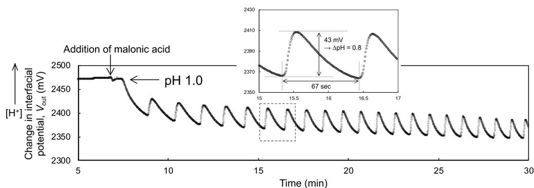
**Figure 1.** Change in interfacial potential ( $\Delta V_{\text{out}}$ ) for BZ reaction detected using single-gate ISFET sensor. Malonic acid was added to the BZ presolution without malonic acid (pH 1.0).  $\Delta V_{\text{out}}$  was translated to pH in accordance with the pH sensitivity of the ISFET sensor (i.e., the Nernstian response) used in this study (Fig. S1).
