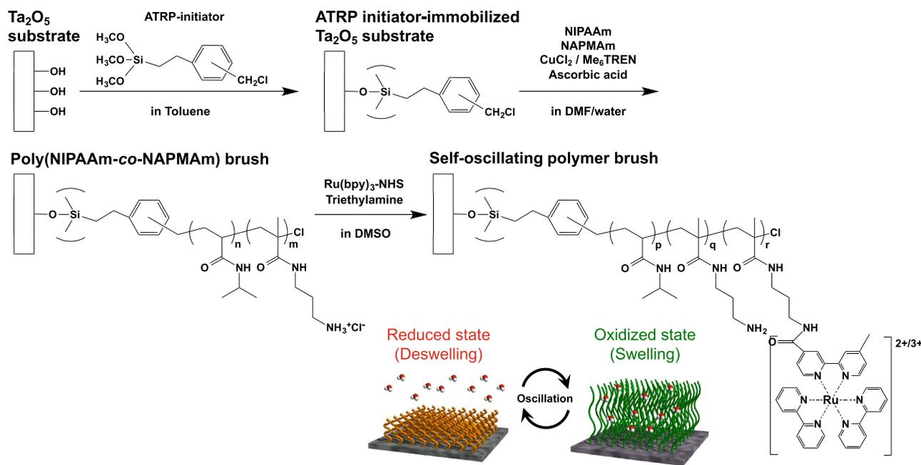
**Figure 5.** Poly(NIPAAm-*r*-NAPMAm-*r*-Ru(bpy)<sub>3</sub> NAPMAm) brush grafted on Ta<sub>2</sub>O<sub>5</sub> gate surface by SI-ARGET ATRP. These illustrations were drawn using the software (ChemDraw ver. 13.0 and Shade 3D ver. 15).
