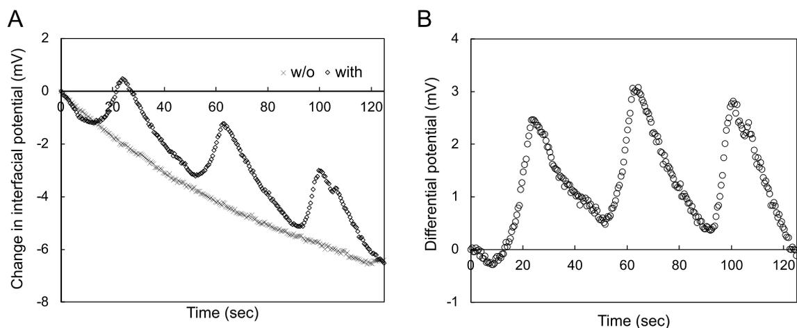
**Figure 6.** Electrical monitoring of self-oscillating polymer brush grafted on Ta<sub>2</sub>O<sub>5</sub> gate insulator using single-gate ISFET sensor. **(A)** Electrical signals for single-gate ISFET sensors with and without self-oscillating polymer brush. **(B)** Differential signal based on **(A)**.
