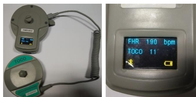
Figure 1: The mobile cardiotocograph device including the probes (FHR and Toco probes)
