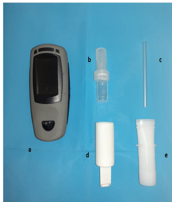
Figure 1 Smokerlyzer's components: electronic device (a); original fitting (b); disposable mouthpieces (c); fitting specially created (d); disposable spirometry mouthpieces (e).
