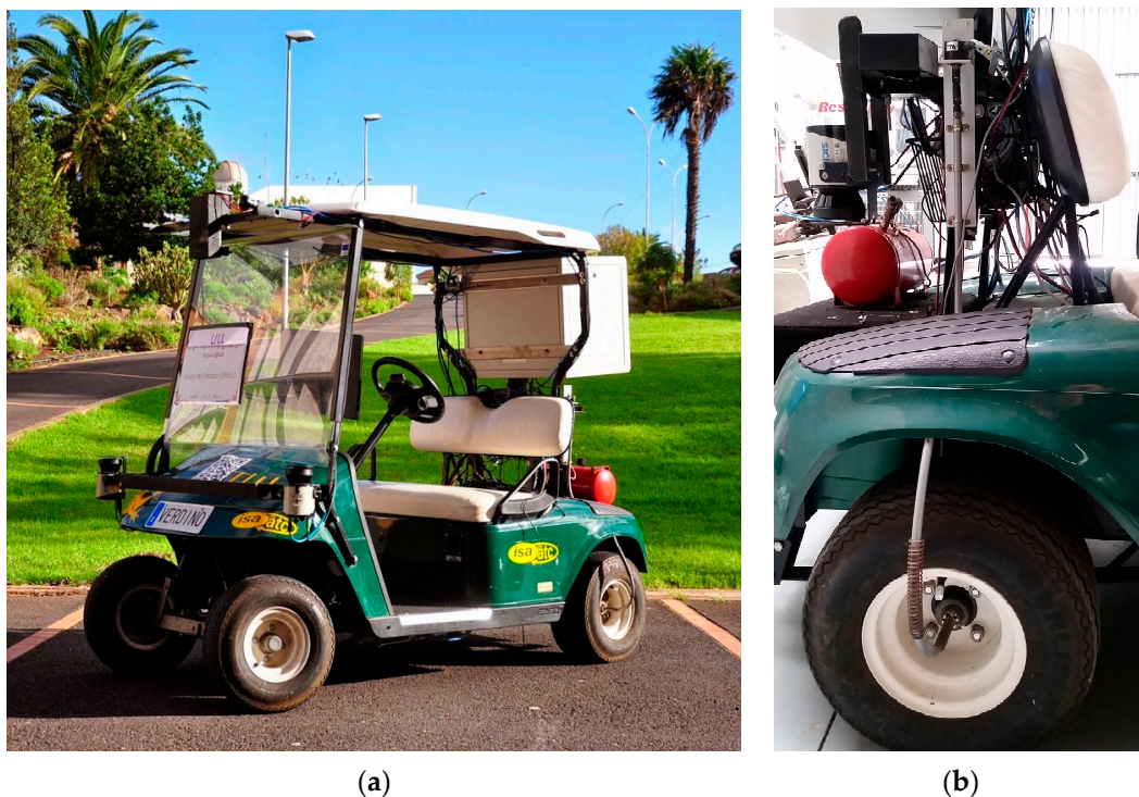
Figure 1. (a) Verdino autonomous golf cart; and, (b) odometric sensor based on a flexible link from the center of the wheel to the encoder placed in the vehicle.
