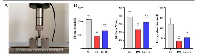
**Fig. 7** Effects of LMHFV on the biomechanical properties of femurs in diabetic rats. **A** Diagram of three-point bending tests at mid-shaft femur sites. **B** The biomechanical properties of cortical bone (e.g. ultimate load, stiffness and energy absorption) are shown in the bar graphs. \*P<0.05, compared with the NC group. P<0.05, compared with the DM group.
