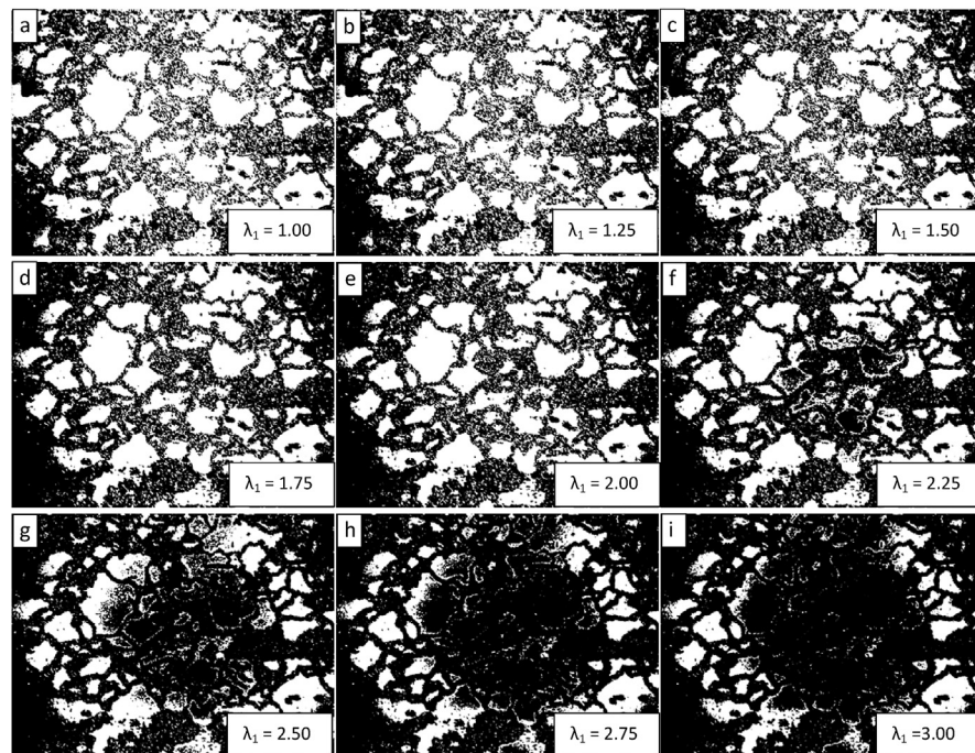
Fig. 10. Demonstration of the convergence of the Chan-Vese algorithm on the image shown in 9 for \mu = 0 , \nu = 0.03 , \lambda_2 = 1.0 , \text{MaxIterations} = 150 , and \lambda_1 varying from 1 to 3 in steps of 0.25 from upper left to lower right (a to i).
