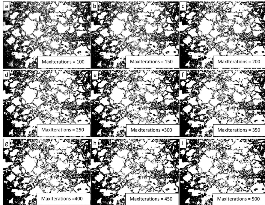
Fig. 11. Demonstration of the convergence of the Chan-Vese algorithm on the image shown in 9 for \mu = 0 , \nu = 0.03 , \lambda_1 = 1 , \lambda_2 = 1.0 , and MaxIterations varying from 100 to 500 in steps of 50 from upper left to lower right (a to i).
