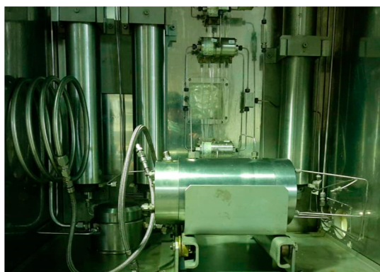
Figure 4. Formation damage and well treatment evaluation system (FDS350) apparatus.
