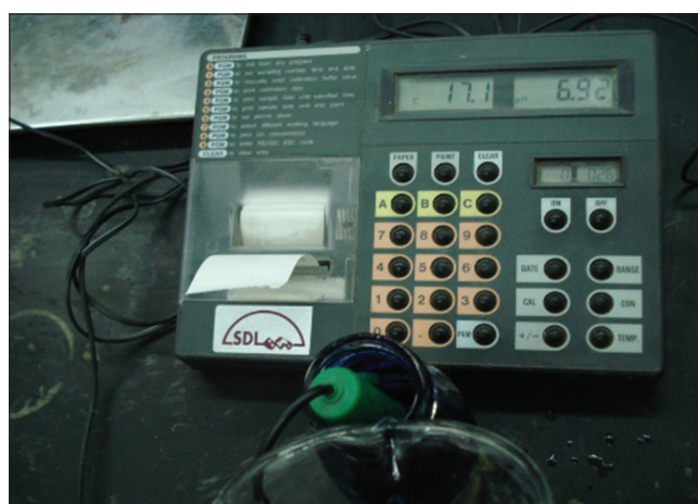
Figure 5: PH Meter Measuring 2 % Methylene Blue after Buffering
