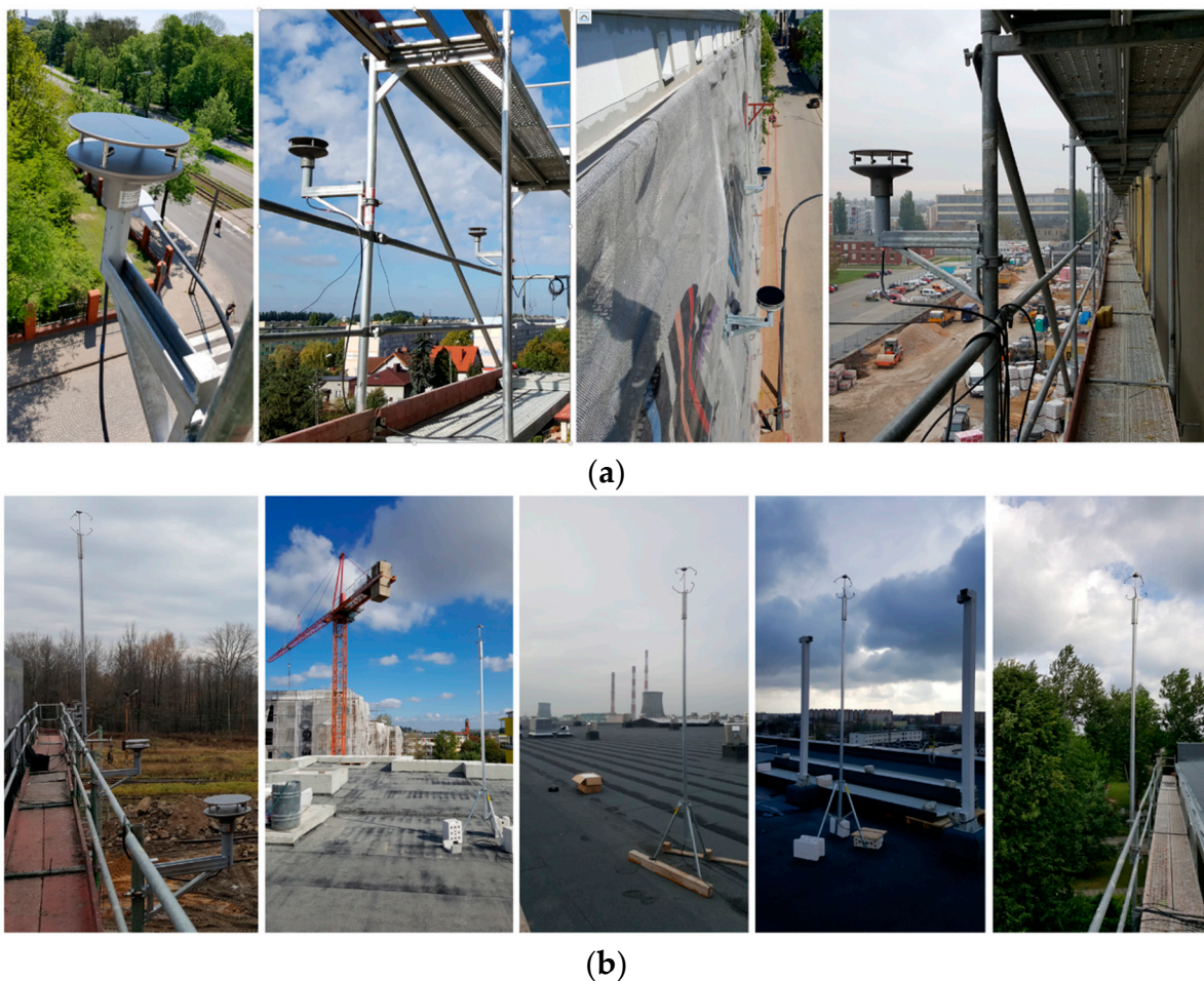
Figure 3. System field application: (a) 2D anemometers; (b) 3D anemometers.
