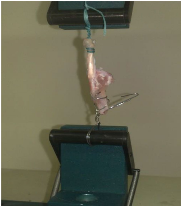
Fig. 1 Biomechanical testing of tendon failure at constant load
