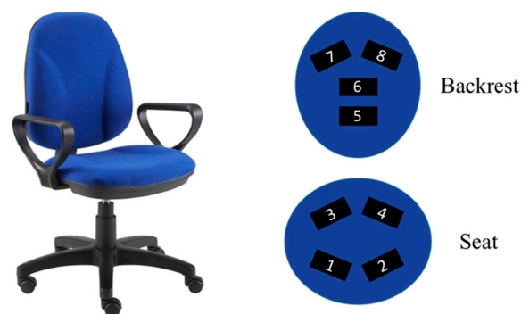
Figure 1. The smart chair and the sensors' position on the chair—analogue tactile pressure sensors (ATSs) 1–4 are located on the seat while ATSs 5–8 are located on the backrest.
