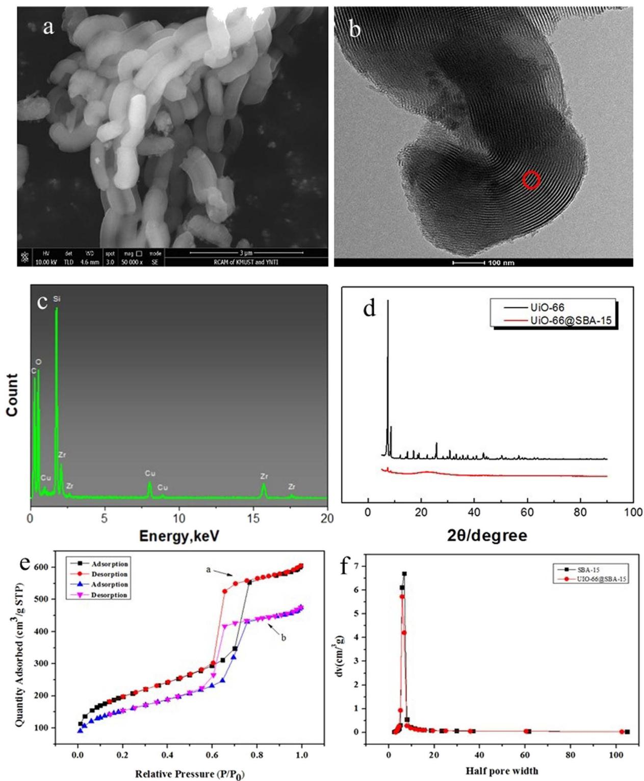
Fig. 2 (a)–(c) SEM and TEM (EDS) images of UiO-66@SBA-15, (d) PXRD patterns of UiO-66 and UiO-66@SBA-15, and (e) and (f) N<sub>2</sub> adsorption isotherms and pore size distribution of SBA-15 and UiO-66@SBA-15.
