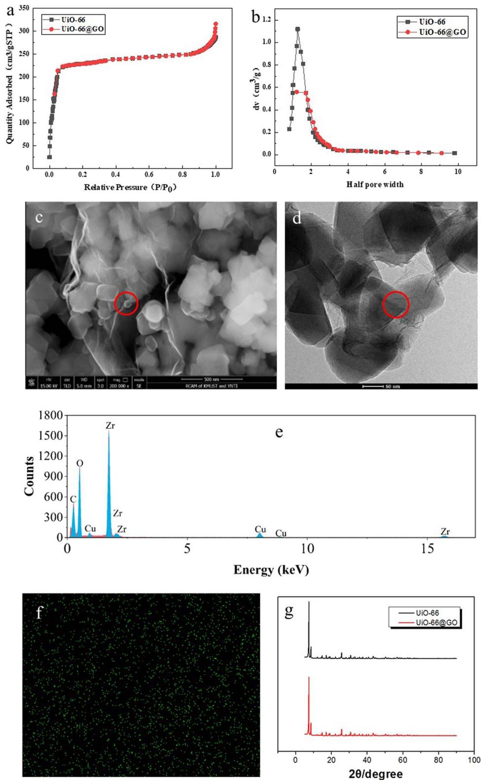
Fig. 3 (a) N<sub>2</sub> adsorption isotherms and (b) pore size distribution, (c) SEM and (d) TEM images of the UiO-66@GO, (e) EDS of the UiO-66@GO, (f) EDX mapping images of UiO-66@GO, and (g) PXRD patterns of UiO-66 and UiO-66@GO.
